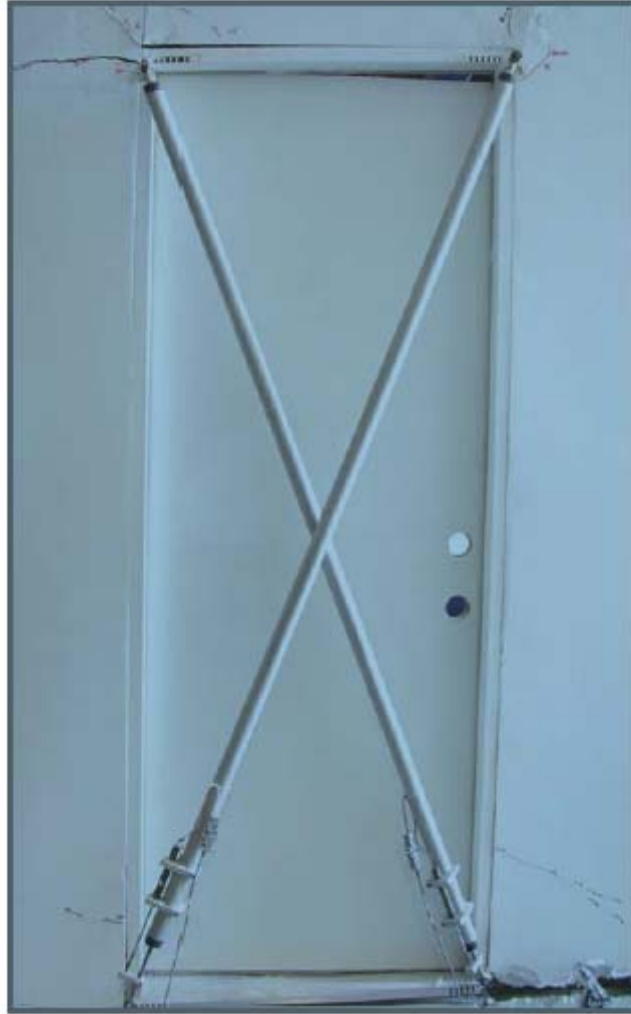
Figure 3. Example of door at large levels of deformation (After Arnold et al.).
